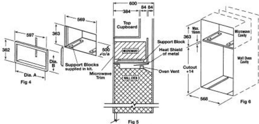
This diagram shows the dimensions that must be used when installing a Microwave above a St George oven.
