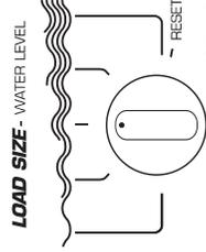
6. Set **LOAD SIZE** (WATER LEVEL) control. Use **RESET** if agitation has started and more water is needed.
